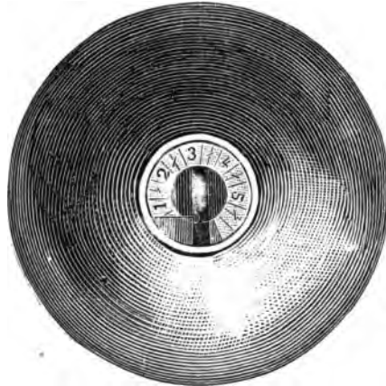
SHELL WITH FUSE.—The fuse is graduated on the outside into equal parts, representing seconds and quarter-seconds. In the bottom of this channel is a smooth layer of a composition of lead and tin, with a piece of wick or yarn underneath it. On this is placed a piece of metal. When ready for firing, the dial is gauged at the proper point at which the fuse is to burn through into the shell.
